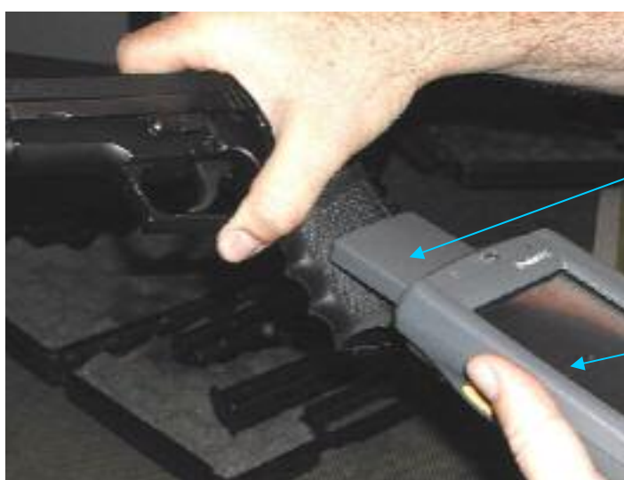
FIGURE 10. Reading the RFID tag fitted in a handgun
