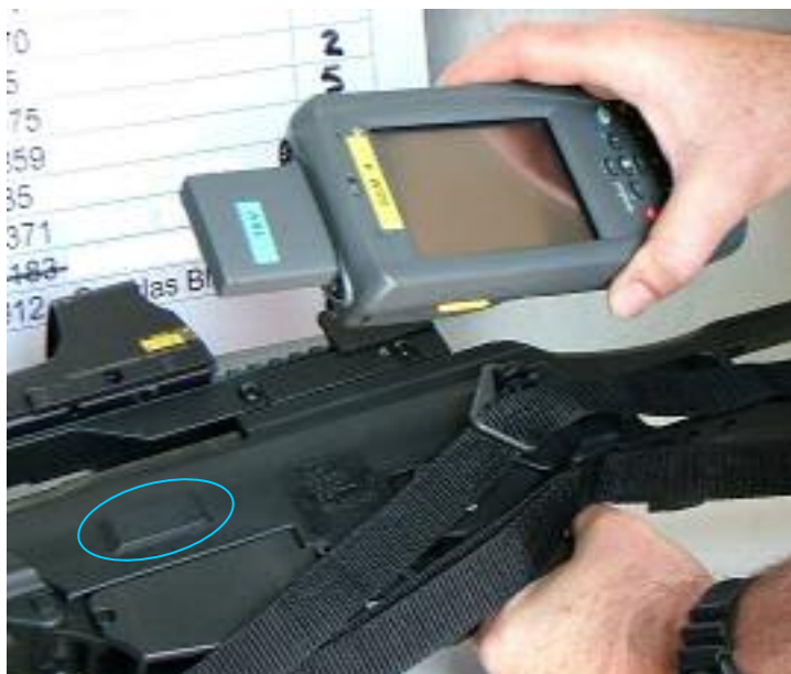
FIGURE 12. Tag fitted to G36
