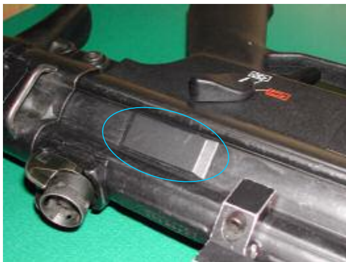
FIGURE 13. Tag fitted to MP5
