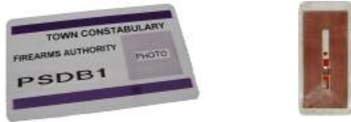
FIGURE 5. RFID tag embedded in a personal identity card and an RFID tag in a laminate form
