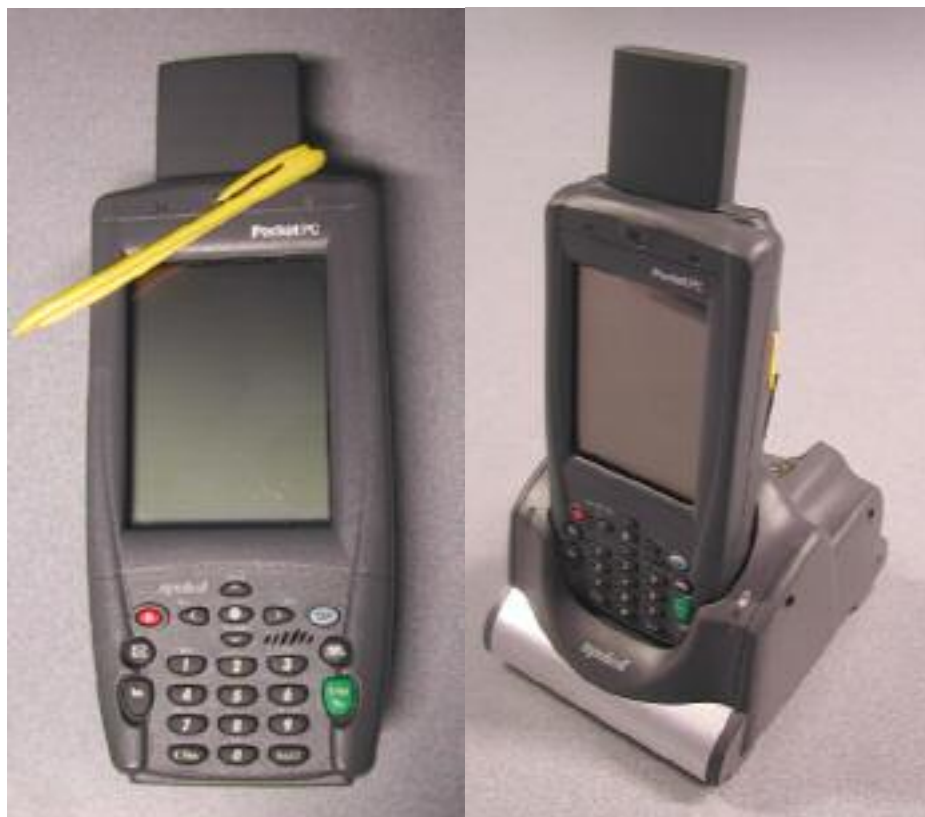
FIGURE 22. Hand-held computer with RFID reader fitted and in desktop cradle
