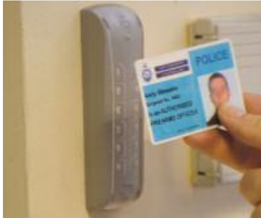
FIGURE 47. Presenting RFID card to door access control reader with keypad
