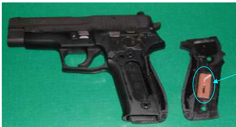
FIGURE 9. Laminated tag fitted under the grip
