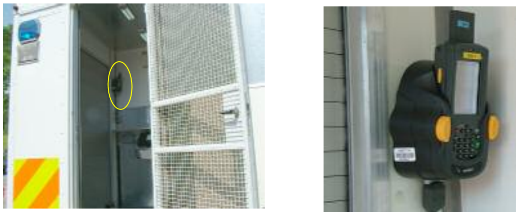
FIGURE 20. Hand-held computer in vehicle mounting cradle fitted in the TSV
