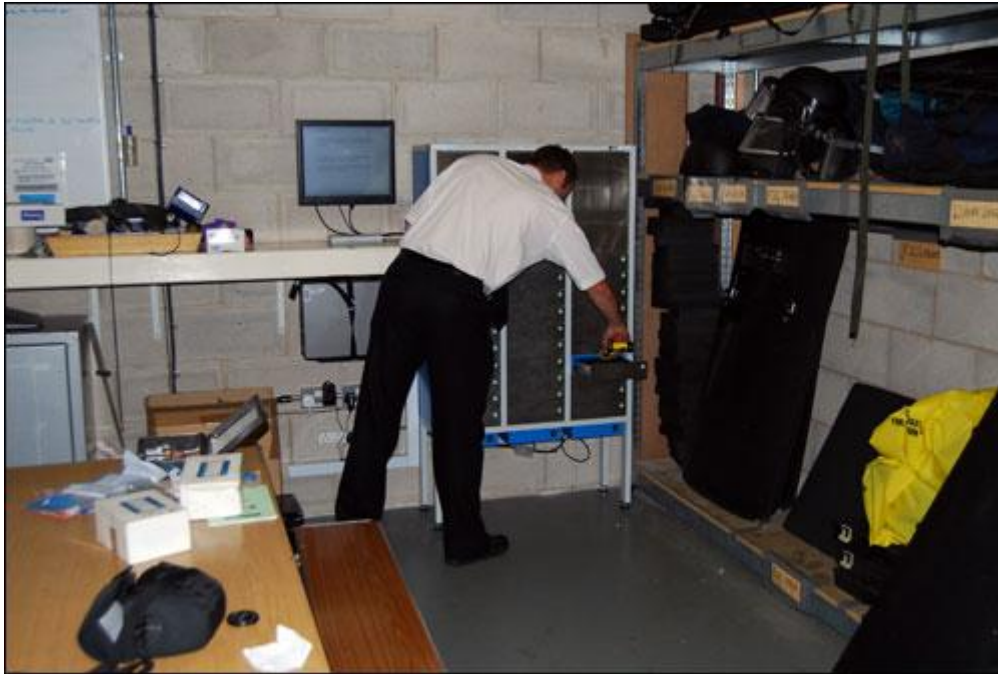
RFID-enabled cabinets were installed to track the condition and usage of Tasers, as well as restrict access.
